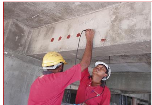
Figure-2 Ultra Pulse Velocity Testing
