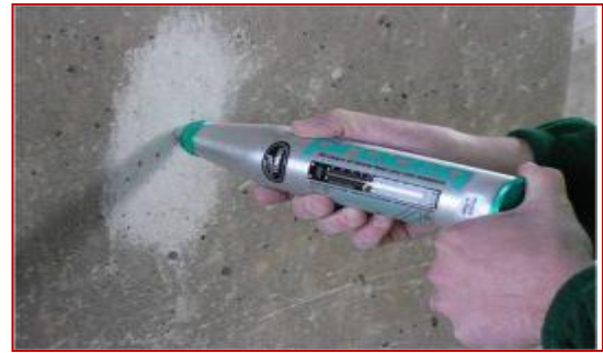
Figure-1 - Rebound Hammer Testing
