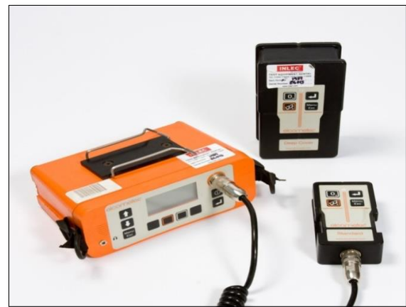
Fig.-4- Bar Locator and Cover Depth Meter
